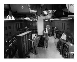
Unlike previous machines, **ENIAC** had no mechanical parts, no counters, and no gears. It relied solely on vacuum tubes. Each vacuum tube contained an electronic circuit, a tiny pathway that carried electricity. Each circuit could turn on and off, much the way a light bulb does.
